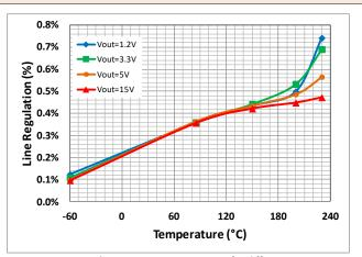
Figure 14. Line Regulation vs Case Temperature for different output voltages.  $I_{LOAD}$ =10mA,  $V_{IN}$  swept from Max[2.8V;  $V_{OUT}$ +0.5V] to 35V.
