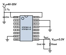
Figure 29. Application of XTR75011 providing 3.3V.
