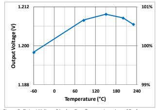
Figure 3. Output Voltage (V\_OUT) vs Case Temperature.  $I_{\text{LOAD}}{=}10\text{mA},$  normalized to  $V_{\text{OUT}}{=}1,2V.$
