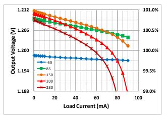
Figure 18. Output Voltage (V\_OUT) vs Load Current for different case temperatures. V\_OUT=1.2V, (V\_IN-V\_OUT)=5V.
