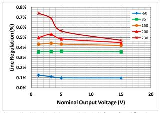
Figure 13. Line Regulation vs Output Voltage for different case temperatures.  $I_{LOAD}$ =10mA,  $V_{IN}$  swept from Max[2.8V;  $V_{OUT}$ +0.5V] to 35V.
