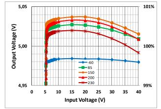
Figure 11. Output Voltage ( $V_{OUT}$ ) vs Input Voltage for different case temperatures.  $I_{LOAD}$ =10mA, normalized to  $V_{OUT}$ =5V.
