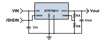
Terminal "XX" represents any terminal from "1.8V" to "15V". In this case the exact output voltage is given by
