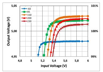
Figure 12. Zoom on the start-up showing Output Voltage ( $V_{OUT}$ ) vs Input Voltage for different case temperatures. I<sub>LOAD</sub>=10mA, normalized to  $V_{OUT}$ =5V.
