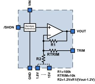
From the block diagram it can be seen that, if the TRIM feature is not used (left floating), the nominal output voltage is given by
