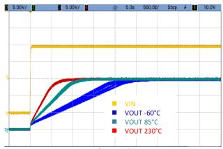
Figure 26. Start-up at V<sub>OUT</sub>=15V for several case temperatures. V<sub>IN</sub> swept from 0V to 20V. /SHDN connected to VIN, C<sub>OUT</sub>=1 $\mu$ F, I<sub>LOAD</sub>=10mA. Overlap of curves from 10 different devices.
