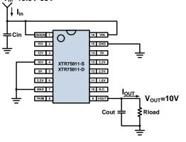
Figure 30. Application of XTR75011 providing 10V.
