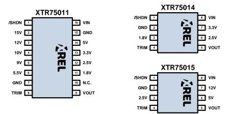
For devices with "FE" package options (CDFP8), ePAD must be connected to VIN.
