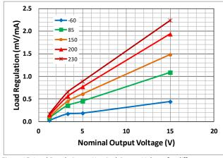
Figure 15. Load Regulation vs Nominal Output Voltage for different case temperatures. Load current sept from 1mA to 30mA,  $(V_{IN}-V_{OUT})=2V$ .
