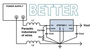
Figure 33. Better breadboard connection with voltage regulator.
