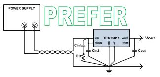
Figure 34. Preferred breadboard connection with voltage regulator.
