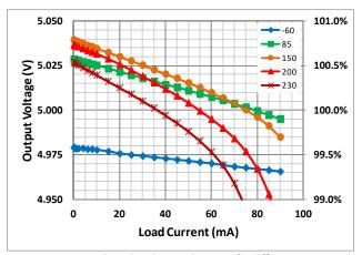
Figure 20. Output Voltage (V\_{OUT}) vs Load Current for different case temperatures. V\_{OUT}=5V, (V\_{IN}-V\_{OUT})=5V.
