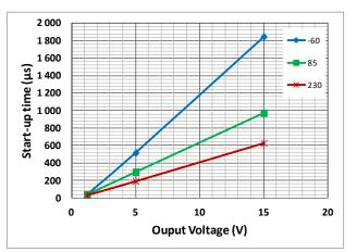
Figure 28. Start-up time vs nominal output voltage for several case temperatures when /SHDN is swept from V<sub>OFF</sub>=0.6V to V<sub>ON</sub>=2.3V with V<sub>IN</sub> constant. C<sub>OUT</sub>=1 $\mu$ F, I<sub>LOAD</sub>=10mA.
