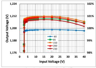
Figure 7. Output Voltage ( $V_{OUT}$ ) vs Input Voltage for different case temperatures. I<sub>LOAD</sub>=10mA, normalized to  $V_{OUT}$ =1,2V.
