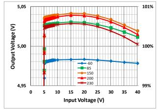
Figure 9. Output Voltage ( $V_{OUT}$ ) vs Input Voltage for different case temperatures. I<sub>LOAD</sub>=0.1mA, normalized to  $V_{OUT}$ =5V.
