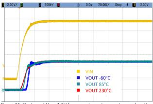
Figure 25. Start-up at V<sub>OUT</sub>=1.2V for several case temperatures when V<sub>IN</sub> swept from 0V to 10V. /SHDN connected to VIN, C<sub>OUT</sub>=1 $\mu$ F, I<sub>LOAD</sub>=10mA. Overlap of curves from 10 different devices.
