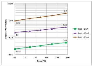
Figure 21. Minimum dropout (V $_{\text{IN}}$ -V $_{\text{OUT}}$ ) vs Case Temperature for different load currents. V $_{\text{OUT}}$ =5V.
