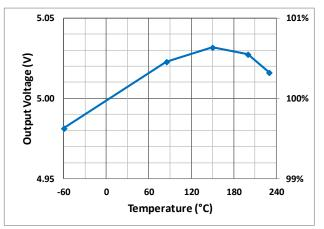
Figure 4. Output Voltage (V\_{OUT}) vs Case Temperature.  $I_{\text{LOAD}}{=}10\text{mA},$  normalized to  $V_{\text{OUT}}{=}5{,}0\text{V}.$
