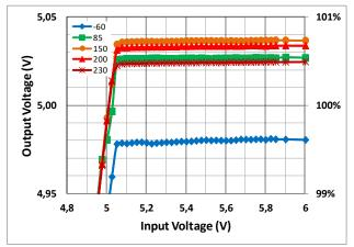
Figure 10. Zoom on the start-up showing Output Voltage (V<sub>OUT</sub>) vs Input Voltage for different case temperatures. I<sub>LOAD</sub>=0.1mA, normalized to V<sub>OUT</sub>=5V.
