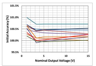
$\label{eq:spectral_spectral} \begin{array}{l} \mbox{Figure 22. Spread of normalized initial output voltage accuracy (V_{OUT-} V_{OUT_Nom})/V_{OUT_Nom} \mbox{ over ten typical samples vs nominal output voltage.} \\ T_c = 85 \mbox{°C, } I_{LOAD} = 1 \mbox{mA and } (V_{IN} - V_{OUT}) = 2 V. \end{array}$
