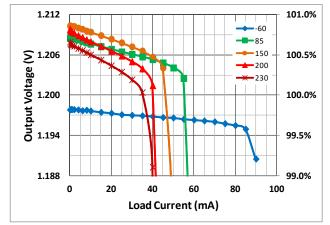
Figure 17. Output Voltage (V\_OUT) vs Load Current for different case temperatures. V\_OUT=1.2V, (V\_IN-V\_OUT)=2V.
