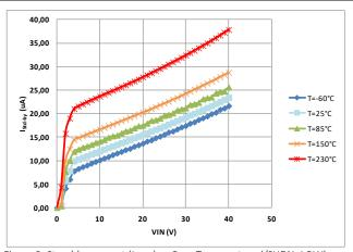
Figure 2. Stand-by current (I<sub>std-by</sub>) vs Case Temperature (/SHDN=LOW).
