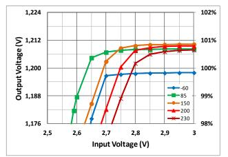
Figure 6. Zoom on the start-up showing Output Voltage ( $V_{OUT}$ ) vs Input Voltage for different case temperatures. I<sub>LOAD</sub>=0.1mA, normalized to  $V_{OUT}$ =1,2V.
