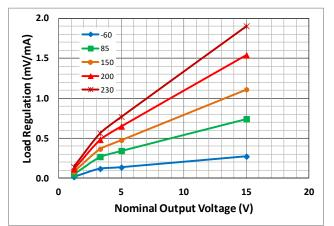
Figure 16. Load Regulation vs Nominal Output Voltage for different case temperatures. Load current sept from 1mA to 50mA, ( $V_{IN}$ - $V_{OUT}$ )=5V.
