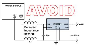
Figure 32. Non-optimum breadboard connection with voltage regulator.
