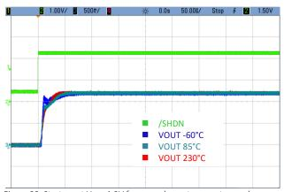
Figure 23. Start-up at V<sub>OUT</sub>=1.2V for several case temperatures when /SHDN swept from 0.5V to 2.3V. V<sub>IN</sub>=10V, C<sub>OUT</sub>=1 $\mu$ F, I<sub>LOAD</sub>=10mA. Overlap of curves from 10 different devices.
