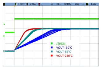
Figure 24. Start-up at V<sub>OUT</sub>=15V for several case temperatures when /SHDN swept from 0.5V to 2.3V. V<sub>IN</sub>=20V, C<sub>OUT</sub>=1 $\mu$ F, I<sub>LOAD</sub>=10mA. Overlap of curves from 10 different devices.
